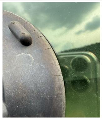
The surface of the ordinary material suction cup shows extensive cracking and aging, with noticeable hardening at the edges. This affects the adhesion function, and its aging resistance is poor, making it no longer suitable for continued use.
