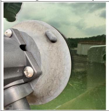
The surface of the suction cup remains in good condition, with no visible cracks or peeling. The functionality is intact, and the appearance is still relatively new, demonstrating excellent weather resistance and stability.
