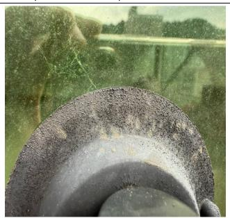
The aging performance of the ordinary material suction cup was poor, with noticeable cracks and severe aging signs:
