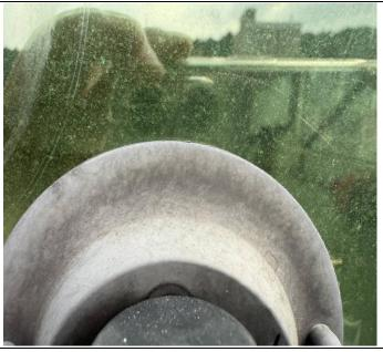
The FSTE well-designed material suction cup demonstrated excellent weather resistance and stability during the 180-day aging test.
